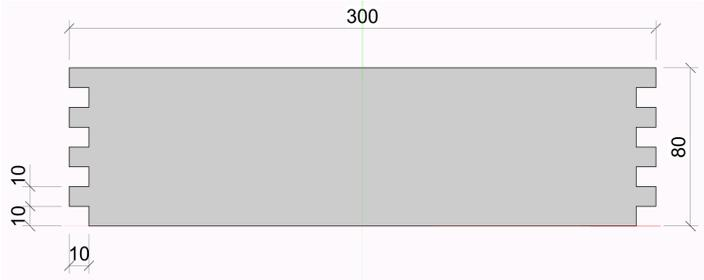
A technical drawing of a rectangular plate with a length of 300mm and a height of 80mm. The drawing shows the front view with finger joints (Fingerzinken) on both the left and right sides. The finger joints are spaced evenly along the length. The drawing includes dimension lines and arrows indicating the 300mm length and 80mm height. The finger joints are shown as a series of rectangular protrusions and recessions.
